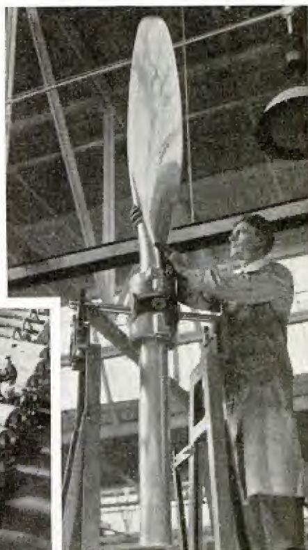
Balancing propeller blade with counterweight to determine the static balance of a propeller
